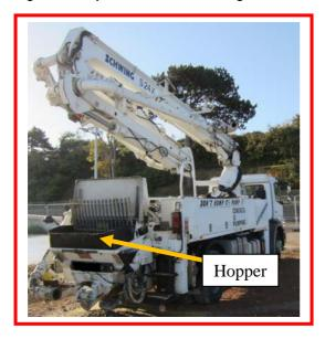
As part of the process of cleaning the pump the driver/operator climbed into the hopper and proceeded to use a lump hammer to loosen hardened concrete from inside the hopper itself. In doing so this caused the turning screw in the bottom of the hopper to re-engage this pulled the operator's foot into the mechanism.
